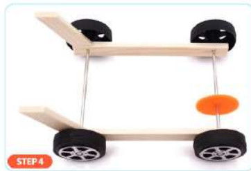
STEP 4 First the gears are mounted on the iron shaft, then the shaft is passed through the frame hole and the wheels are mounted
