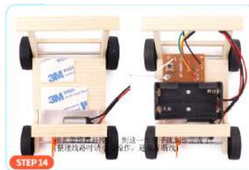
STEP 14 Glue the two double-sided tapes to the positions shown on the picture. Attach the battery box and the receiving plate to the double-sided adhesive tape, and pay attention to the directions of the accessories in the picture above. Do not use hot melt adhesive to fix the circuit board, otherwise it will cause short circuit of electronic components!
