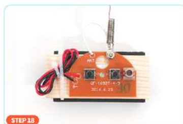
STEP 18 Glue the battery box and the remote control board to the board separately. Tie up the wiring (to avoid breakage). Remote control finished!
