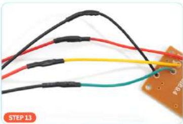
STEP 13 After the wire is connected, move the black heat-shrinkable tube to the wiring area, heat the heat-shrinkable tube with a lighter to shrink, and seal the wiring area.
