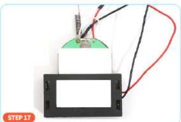
STEP 17 Attach a double sided adhesive tape to the back of the remote control board and the back of the battery box
