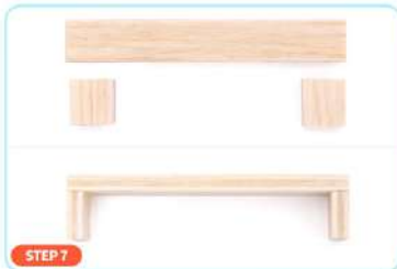
STEP 7 First prepare the parts of the motor bracket, and then glue them together (When bonding, please note that the grain direction of the square block in the figure above must be the same, if not, it will lead to a high side and a low side)
