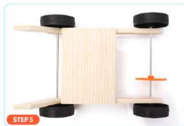
STEP 5 Glue the wide wooden block to the frame, glue the wide wooden block to align the back end and both sides, do not exceed, do not stick crooked. When viscose water pay attention to the glue do not permeate the wheel shaft hole
