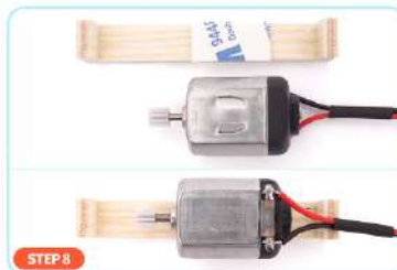
STEP 8 First on the motor bracket with the appropriate size of double-sided adhesive tape, and then the motor to the support frame
