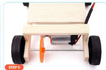
STEP 9 Install the motor module on the frame, gear must be on, if not, please first adjust the big gear to the right position, until the two gear match. To be glued together. (if the gear does not fit too tight, the transmission resistance will be great, which may lead to the failure of rotation)
